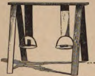
FIG. 84.—Device to illustrate the different effects upon the transmission and the character of shocks which are produced by firm rock and by loose materials.
